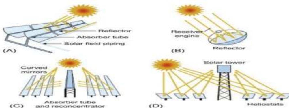
Figure 5: Concentrated Solar Power Plant [3]
